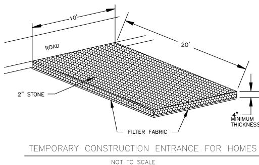
PLAN SHOWING CONSTRUCTION SEQUENCING EROSION AND SEDIMENT CONTROL NARRATIVE AND DETAILS
