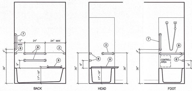
4 HANDICAP BATHROOM ELEVATIONS
