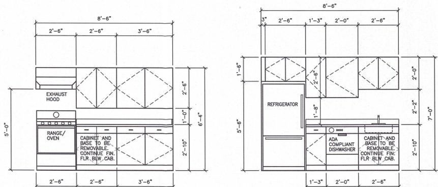
7 UNIT 2 KITCHEN ELEVATIONS HANDICAP ADAPTABLE
