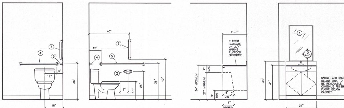
5 HANDICAP LAVATORY SECTION/ELEVATION
