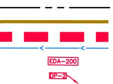
PROPERTY LINE EXISTING SOIL BOUNDARY EXISTING DRAINAGE BOUNDARY EXISTING TIME OF CONCENTRATION EXISTING DRAINAGE AREA ID EXISTING DESIGN POINT
