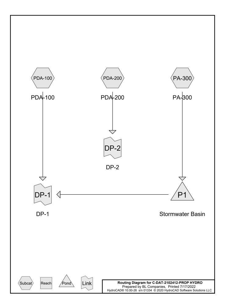
Time span=0.00-30.00 hrs, dt=0.01 hrs, 3001 points Runoff by SCS TR-20 method, UH=SCS, Weighted-CN Reach routing by Stor-Ind+Trans method - Pond routing by Stor-Ind method
