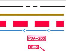
PROPERTY LINE PROPOSED SOIL BOUNDARY PROPOSED DRAINAGE BOUNDARY PROPOSED TIME OF CONCENTRATION PROPOSED DRAINAGE AREA ID PROPOSED DESIGN POINT
