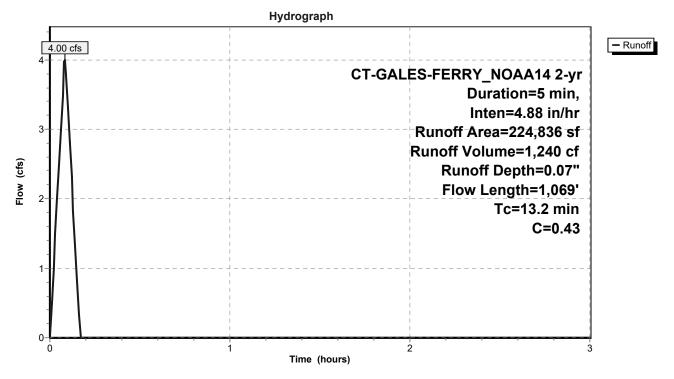
C-DAT-2102412-PROP HYCT-GALES-FERRY\_NOAA14 2-yrDuration=5 min,Inten=4.88 in/hrPrepared by BL CompaniesPrinted 7/26/2022HydroCAD® 10.00-26 s/n 01334 © 2020 HydroCAD Software Solutions LLCPage 5
