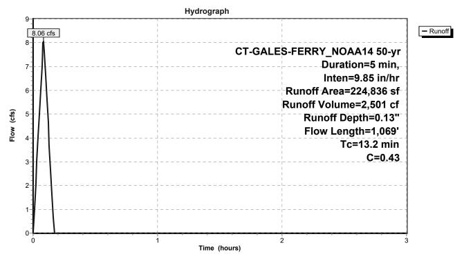
C-DAT-2102412-PROP HYCT-GALES-FERRY\_NOAA14 50-yr Duration=5 min, Inten=9.85 in/hr Prepared by BL Companies Printed 7/26/2022 HydroCAD® 10.00-26 s/n 01334 © 2020 HydroCAD Software Solutions LLC Page 17
