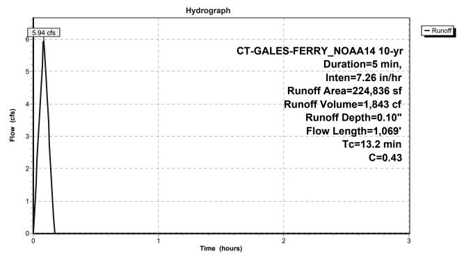
C-DAT-2102412-PROP HYCT-GALES-FERRY\_NOAA14 10-yr Duration=5 min, Inten=7.26 in/hr Prepared by BL Companies Printed 7/26/2022 HydroCAD® 10.00-26 s/n 01334 © 2020 HydroCAD Software Solutions LLC Page 9
