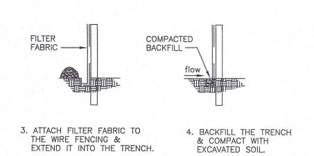
FILTER FABRIC SEDIMENT BARRIER
