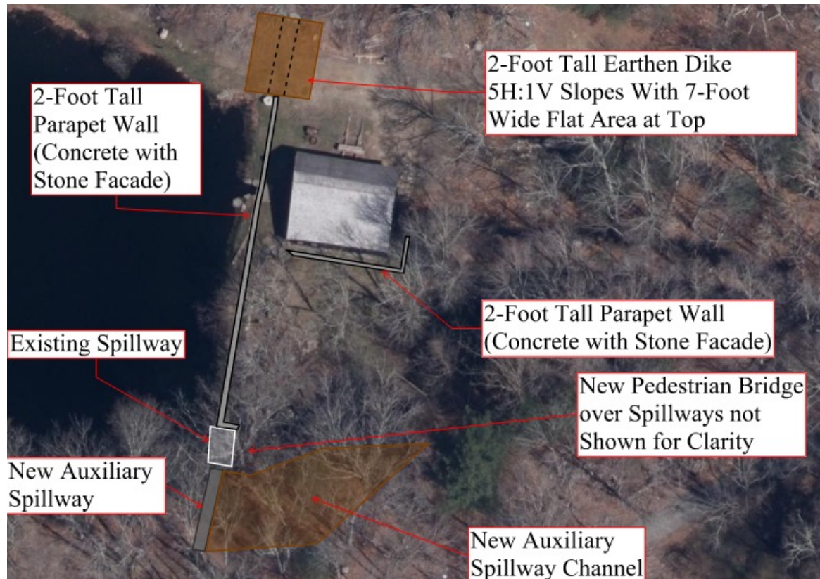
Figure 2- Conceptual Alternative No. 2 Rehabilitation- Auxiliary Spillway
