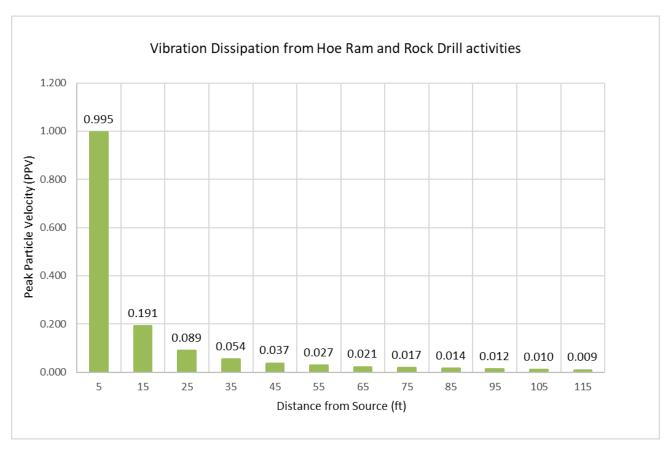
Additionally, using this calculation process, the closest construction activity to each location was used to calculate worst-case vibration calculations for each location. While these charts include all of the equipment in the standard FTA calculations, the highest vibration generation anticipated from this site is highlighted in green.
