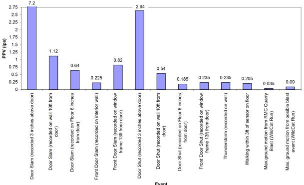
Proper construction and maintenance can minimize these effects, but it is impossible to eliminate all of the effects brought about by environmental changes. Environmental changes and normal household activities cause more stress on a structure than typical vibration levels from typical construction and regulated blasting activities.
