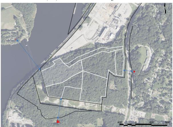
Measurements on the aerial image above show the closest distance from each of the off-site locations to any of the blasting operations. These distances, 22 Anderson Drive (260 ft), 40 Chapman Lane (562 ft) and 89 Point Breeze Road (1,018 ft), are used for our calculations below.
