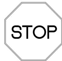
SECURE TO 1 1/2" GALVANIZED STEEL POST WITH (2) 1/4" GALVANIZED BOLTS (1 TOP, 1 BOTTOM)
