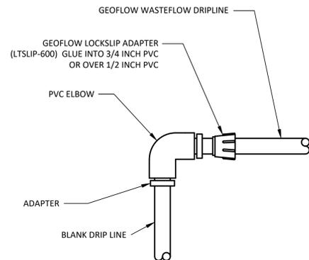
MANIFOLD ELBOW CONNECTION
