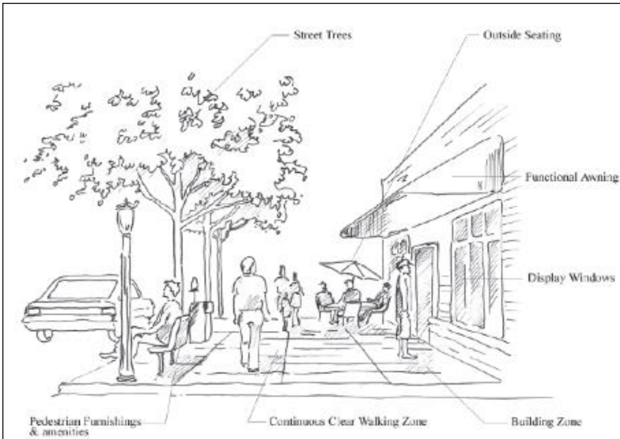
Streetscape. Source: Design Guidelines for the Village of Watkins Glen prepared by Synthesis.
