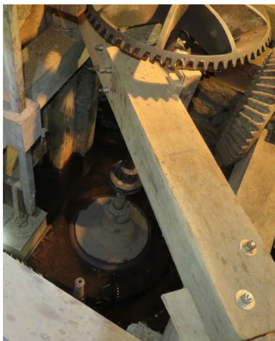
Left: 1870 advertisement for the Tyler Turbine; Right: Top of turbine in-situ.
