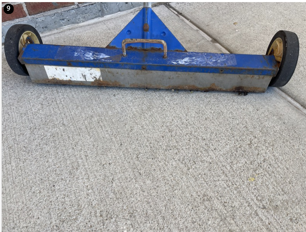
9 The crew actively combing the area for nails with the magnet cart
